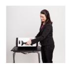
Stand at the front of the booth. Reach under the front of the booth top and push the latch away from you to secure the Touch Writer to the booth.
