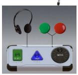
**Verity Touch Writer Duo** may be used with **Verity Access**, an Audio-Tactile Interface (ATI) intended for voters that cannot, or prefer not to, use the touchscreen. Verity Access includes two connection ports: the left connection port for headphones, and the right connection port for any dual-switch input device (such as tactile switches or sip-and-puff devices). For more information, see page 27.
