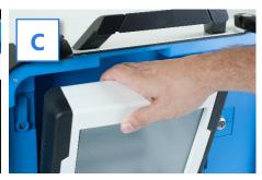
9. Seat the tablet in the cradle (A), tilt it back (B), and lock it in place (C). ▼
