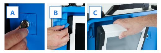
9. Seat the tablet in the cradle (A), tilt it back (B), and lock it in place (C).
