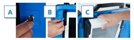
8. Seat the tablet in the cradle (A), tilt it back (B), and lock it in place (C).▼
