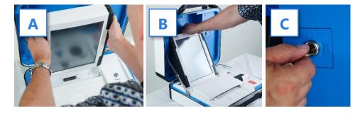
Verify the Verity Scan device seals, per local procedure. Attach privacy screens to each side of the ballot box, if applicable. ►
