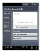
6. Wait while the Access Code prints on Verity Controller's built-in thermal printer. Hand the printed Access Code to the voter and direct them to the Verity Touch booth.
