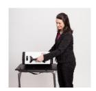
2. Stand at the front of the booth. Reach under the front of the booth top and push the latch away from you to secure the Touch Writer to the booth.
