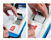
4. Close the printer cover. The paper must extend out from underneath the front edge of the cover. The white button can be used to advance the paper.
