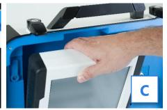
8. Seat the tablet in the cradle (A), tilt it back (B), and lock it in place (C). ▼
