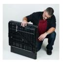
2. Unlatch the four clips (two on each side).
