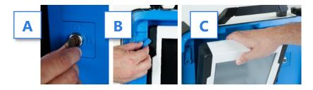
9. Seat the tablet in the cradle (A), tilt it back (B), and lock it in place (C). ▼
