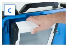
9. Seat the tablet in the cradle (A), tilt it back (B), and lock it in place (C). ▼
