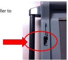
**6.** Unlock the back panel on the Duo Go carrier and open the back panel door (removing the tamper seal first, if applicable).
