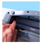
8. Connect the USB cable on the inside of the Duo Go carrier to the port on the side of the tablet. A tamper seal may be used to secure the cable; remove this seal first, if applicable.
