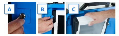
6. Seat the tablet in the cradle (A), tilt it back (B), and lock it in place (C). ▼
