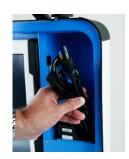
3. Plug the power cord into the power brick, and then plug the power brick into the back of the Verity Controller (flat side up). ▼
