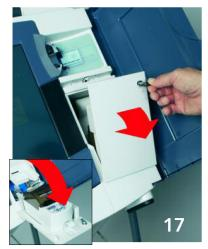
Use key to open printer access door and swing it down.
