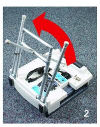
Gripping the black handle, pull the support bar away from the base. Remove the power cord, keypad and headset from the back of the unit as applicable.
