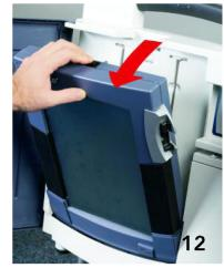
To set up a Visually Impaired Ballot Station (VIBS) unit press on the tablet's black notch and pull the tablet forward. If you are **NOT** setting up a VIBS unit, go to step 15.
