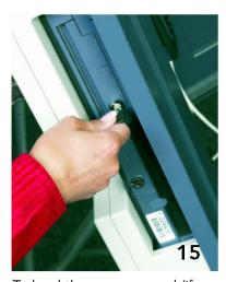
To load the memory card (if applicable), unlock the memory card door on the unit's left edge.
