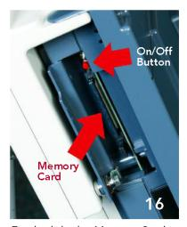
Firmly slide the Memory Card in place as shown. Turn on the unit's power, then close and lock the door.
