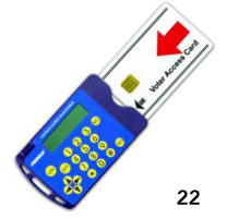
Insert the Voter Access Card into the encoder with the gold chip facing you and press "ON".
