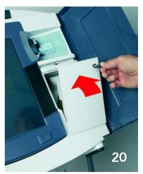
Close printer access door and lock with key.
