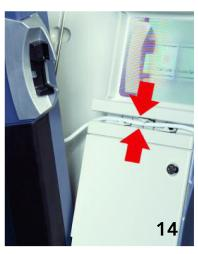
Place the tablet back into its cradle and feed the cord through the mounting slot. Set the keypad aside.
