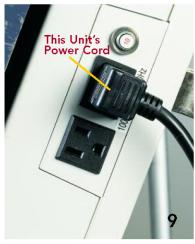
If you are only setting up one TSX, go to step 12. Otherwise, take the power cord from the first unit and plug it into an outlet. Attach the female end to the top socket.
