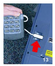
Pull the tablet out of the cradle. and plug the keypad into the port on the back.
