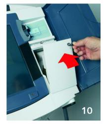
Close the printer door and lock it. Disconnect power cord, headset and keypad from the tablet (if applicable). Remove keypad from mounting slot.
