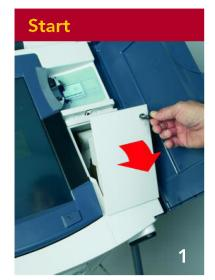
Use key to open printer access door and swing it down.
