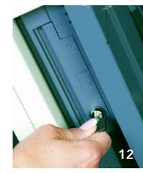
Verify the memory card slot is locked and seal if mandated. Turn the unit upside down and place it on its face.
