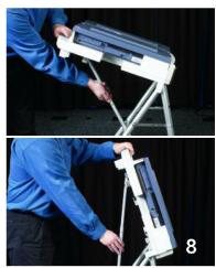
To adjust the angle, lift up on the handle while pressing the safety pin on the support bar.
