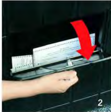
If any uncounted ballots were dropped in the lower door, remove them and handle per instructions from your local election office. Uncounted ballots may be processed through the AccuVote unit at this time.
