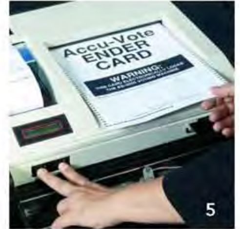
Locate the ENDER Card. Press and hold the YES and NO buttons at the same time. While holding the two buttons, insert the ENDER CARD into the AccuVote unit.
