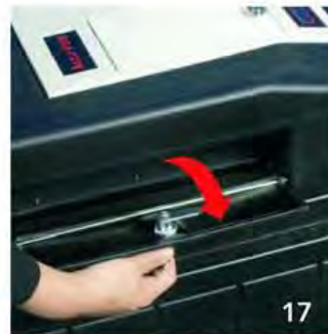
17 In the instance the AccuVote unit fails, unlock the top left side door on the ballot box using the brass key with plastic key cap. Direct voters to deposit voted ballots into this slot and call your assigned support team for further instructions.
