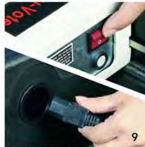
Turn off the AccuVote unit by pressing the red ON/OFF switch on the back of the unit. Unplug the power cord from the wall, then unplug the unit and remove the power cord. Repack the unit in its case.
