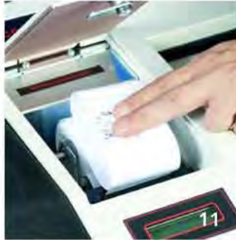
11 When all necessary reports have been printed and been signed, fold or roll at least one report and place it in the printer compartment.
