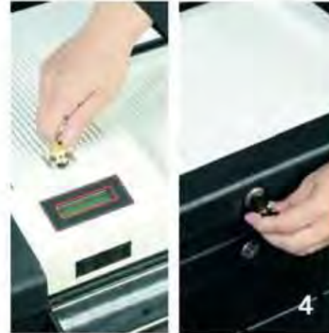
Unlock and remove the printer cover using the plain brass key. Unlock and open the retaining door of the ballot box using the brass key with plastic key cap.
