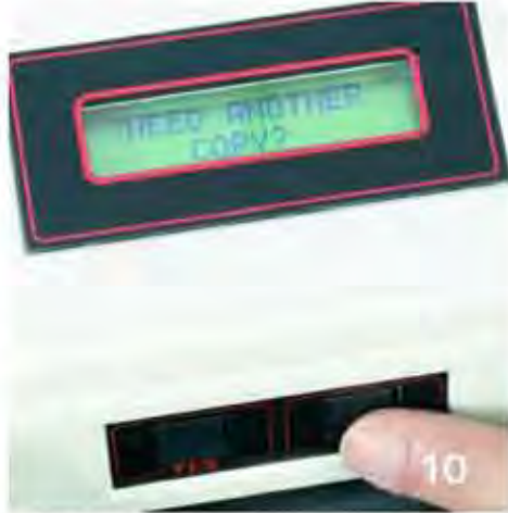
10 The LCD Screen on the AccuVote Unit will display, "NEED ANOTHER COPY?" Push YES to print an additional copy and then push NO when prompted again.
