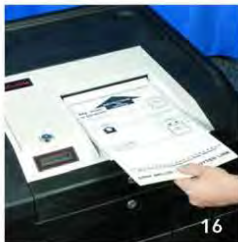
16 When a voter completes their ballot, the ballot should be inserted into the AccuVote unit like a dollar bill changer. The ballot is tallied and pulled into the ballot box.
