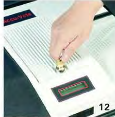
12 Replace the printer cover and using the plain brass key, lock the printer.
